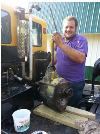
Tyler Vadney removed the transmission on the Bombi for a rebuild Sept 17th. Skip Murrell has been volunteering his time to work on the hydraulic and electrical systems.
