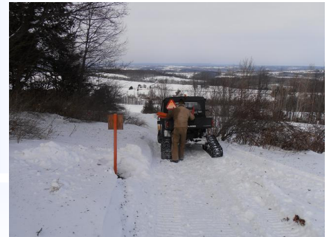
Laudy's side by side works not only as a groomer but also carries sign posts, a generator, and tools for putting in the posts.
