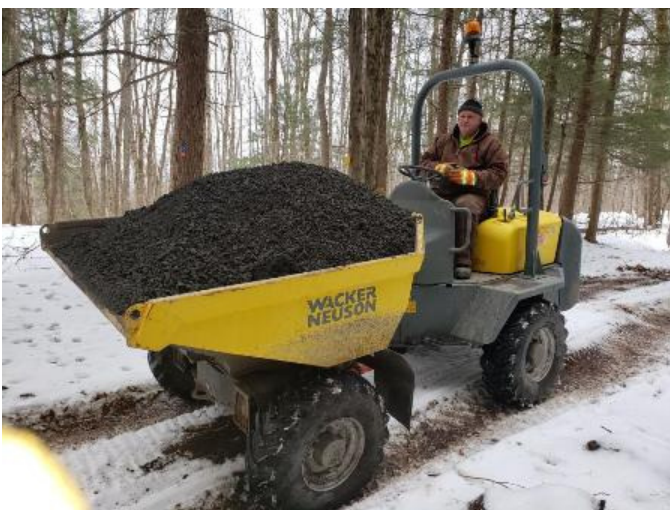
An articulated ATV rock truck brings in a load of shale. Photos by Gerry Lenseth
