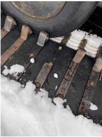
Broken track guide on Bombi.
