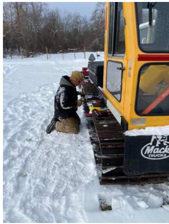
Skip Murrell replaces broken track guide.
