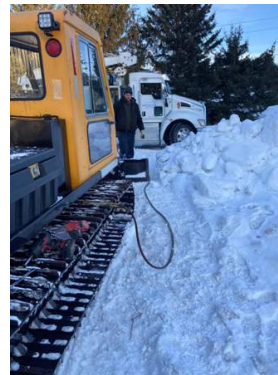
Bombi having some broken track clips replaced.
