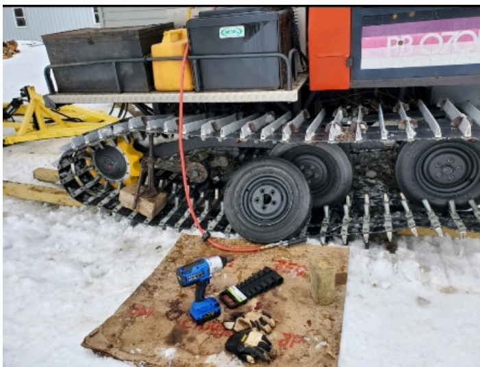
The Pisten Bully 70 suffered 2 flat tires after many hours of grooming. Here it is being repaired in Esperance by Tom Rulison. Cold weather makes outdoor repairs challenging.
