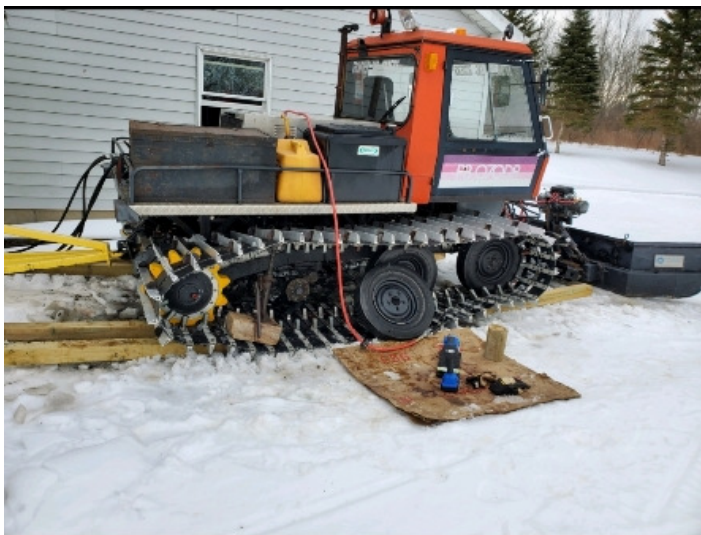
The Pisten Bully 70 suffered 2 flat tires after many hours of grooming. Here it is being repaired in Esperance by Tom Rulison. Cold weather makes outdoor repairs challenging.
